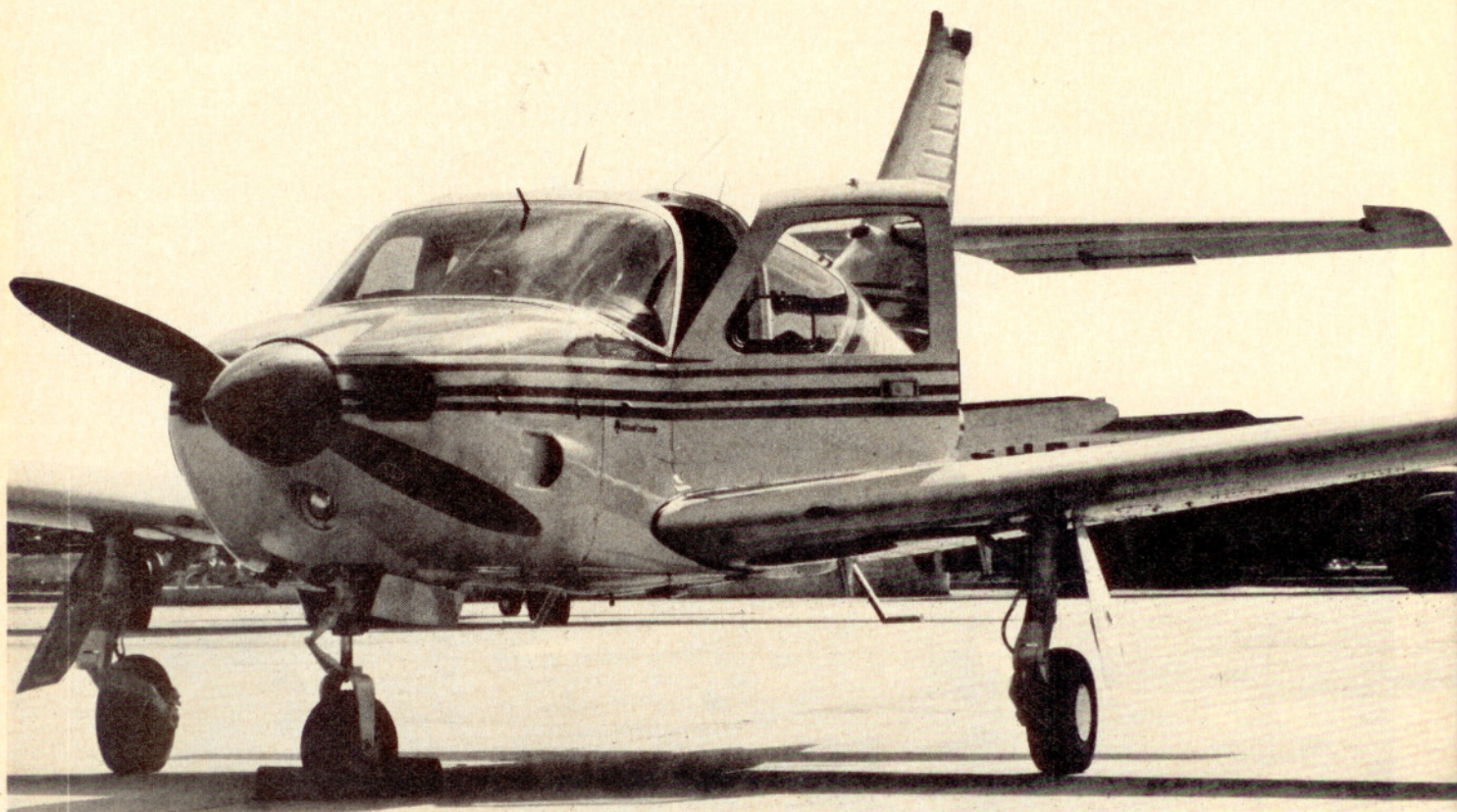
Trailing beam landing gear design has always provided for "cushy" landings. Photos by the author.
